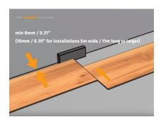
5. To install the next row simply place the new element in the long groove of the previously installed row at an angle of around 30° and lower it into place. The short profile is locked into place after lowering.
