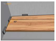
4. The first element - tongue side always adjacent to wall - is laid. The second and following elements should then be slid into place flat and horizontally.
