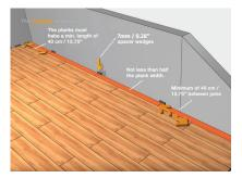
9. The locking system ensures a high, point and reliably prevents the join on the short profile springing out.
