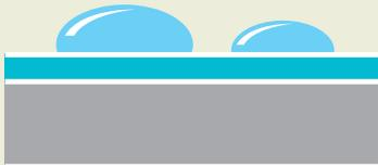
The **EVERCARE™** water-repellent effect prevents staining products from penetrating the materials (alcohol-based Eosin and Betadine, hydro-alcoholic gels, etc.), remaining on the surface.
