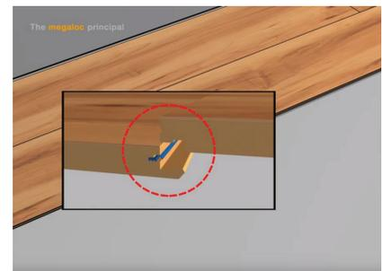
6. The locking system ensures a high, point and reliably prevents the join on the short profile springing out.
