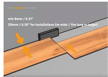
5. To install the next row simply place the new element in the long groove of the previously installed row at an angle of around 30° and lower it into place. The short profile is locked into place after lowering.
