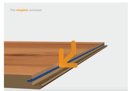
2. Isowaxx® is pressed between the joints automatically during installation sealing it at the same time.
