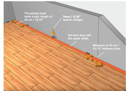
9. The locking system ensures a high, point and reliably prevents the joint on the short profile springing out.
