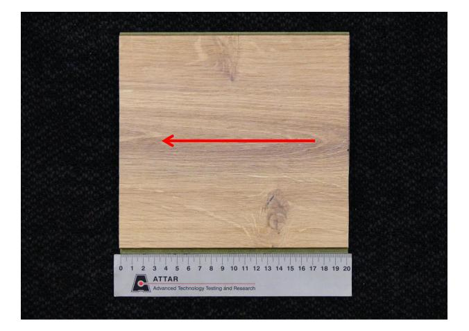
Figure 1:Finfloor Original - Tibet Finish<br/>Arrow indicates direction of testing
